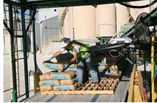
Worker performing manual materials handling while palletizing 100 pound bags of sand.
